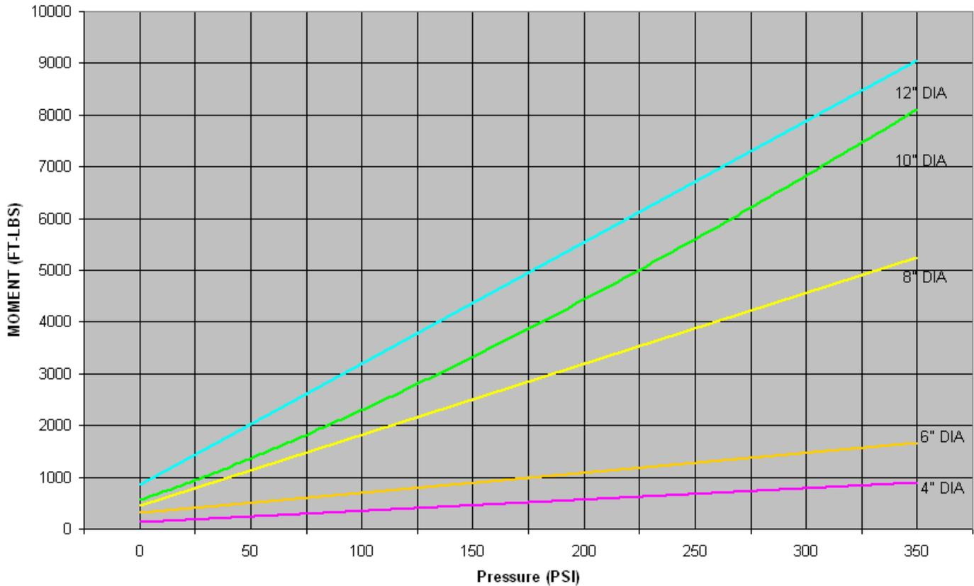
The graphs above represent the bending moments required to rotate the ball joint of Flex-Tend flexible expansion joints at various hydrostatic pressures, 4 through 12 inch nominal sizes. The data for these curves was gathered through deflection load analysis of full scale production models of each size. Deflection moments were measured for pressures ranging from 0psi through 350psi in increments of 50psi.
