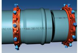
The Series 2916 is designed for restraining AWWA C909 PVC Pipe with push-on bells. It has one restraint ring behind the bell and on the plain end.
