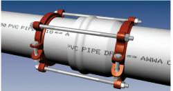
6. Place nuts on the tie bolts and tighten until they are snug. Allow enough room on the tie bolt to fully engage the nut with several threads showing. Do not tighten these bolts enough to force the spigot further into the bell of the joint.
