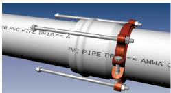
4. Remove the side bolts from the serrated restraint ring. Use the tie bolts to determine the proper location of the restraint ring on the spigot. Allow enough room on the tie bolt to fully engage the nuts.
