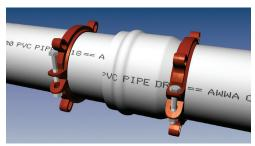
5. Install both halves of the restraint ring at the proper location, tapping each half into place. Make sure that the complete ID of the ring is touching the pipe before installing the side bolts. Tighten the side bolts evenly to 60 ft-lbs torque (110 ftlbs on 8 inch, 10 inch and 12 inch).
