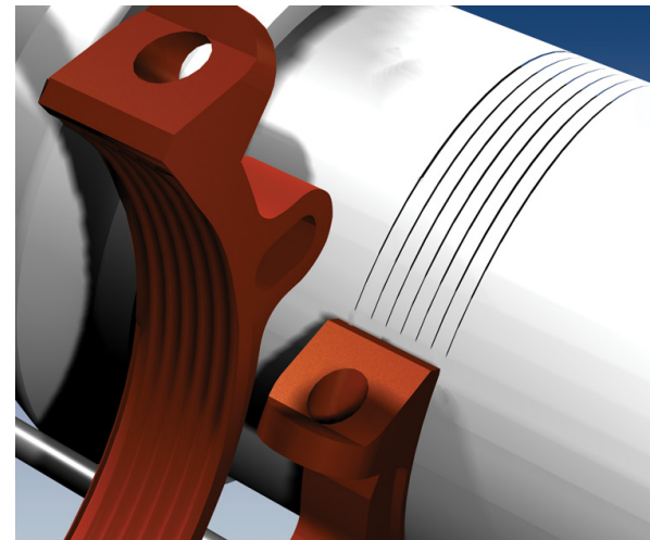
Restraint Ring Tooth Impressions on PVC Pipe.
