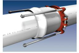
4. Remove the side bolts from the second serrated restraint ring. Use the Thrust Bolts to determine the proper location of the restraint ring on the spigot. Allow enough room on the thrust bolt to fully engage the puts
