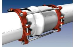
Place nuts on the thrust bolts and tighten until they are snug. Allow enough room on the thrust bolts to fully engage the nuts. Do not tighten these bolts enough to force the spigot further into the bell of the joint.
