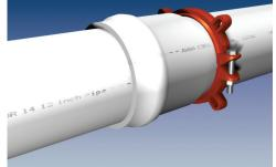
3. Install both halves of the serrated ring around the pipe behind the bell, tapping each half into place. Make sure that the complete ID of the ring is touching the pipe before installing the side bolts. Install the side bolts and tighten evenly to 110 ft-lbs. of torque. (60 ft-lbs on 4 inch and 6 inch)
