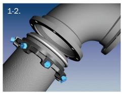
1. The Series 1100 MEGALUG® joint restraint is designed for use on ductile iron pipe conforming to ANSI/AWWA C151/A21.51 (all thickness classes) when restraining mechanical joint pipe fittings.
