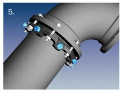
sizes (30 through 64-inch [762mm – 1,600mm]), five or more repetitions may be required. The use of a torque-indicating wrench will facilitate this procedure.
