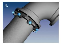
Improved Mechanical Joint Gasket, there is no narrow end as the gasket is bi-directional. In certain sizes, use of the EBAA-SEAL is required to achieve the pressure ratings of the MEGALUG.] NOTE: In cold weather it is preferable to warm the gasket to facilitate assembly of the joint.
