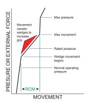
of the pocket at the maximum pressure or load, the wedge buttress are in shear. The maximum movement is about 0.3 inch through the thirty-six inch size and 0.4 inch for forty-two and forty-eight inch. The RCM is available even with severe cyclic loads. This has been tested to very high-pressure differentials and the wedge impressions look the same as if a single test had been performed.
