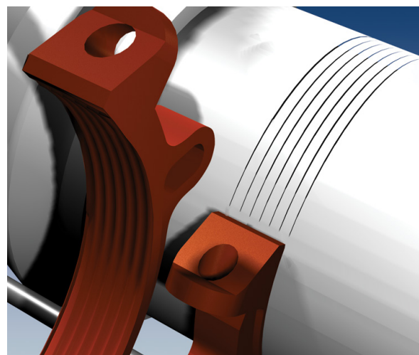
Restraint Ring Tooth Impressions on PVC Pipe.
