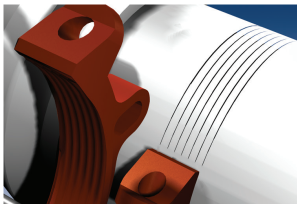
Restraint Ring Tooth Impressions on PVC Pipe.
