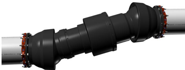
This dual-acting cylinder scenario schematically describes the design of the FBFT. It has a primary cylinder (the same one that exists with the standard FT) but it also has a secondary cylinder. In operation, the hydraulic source is the fluid in the pipeline. Each cylinder has the same hydraulic area and is pressurized by the same source. As a result, the **force** from each cylinder is **balanced**.
