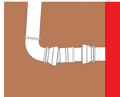
The expansion portion of the FT, the primary cylinder, acts like a conventional, single-acting hydraulic cylinder which is free to move within its physical limits. The following diagram illustrates how a FT, located between a bend (on the left) and a fixed structure such as a building (on the right) can affect the adjacent piping once the piping is pressurized and the thrust force comes to bear.
