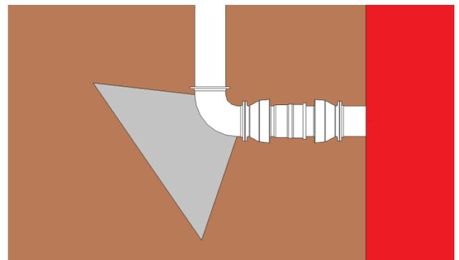
In order to accommodate the thrust force a physical restraint (in this example, a thrust block) must be incorporated into the design to keep the thrust force in check while allowing the FT to move freely when differential movement occurs.
