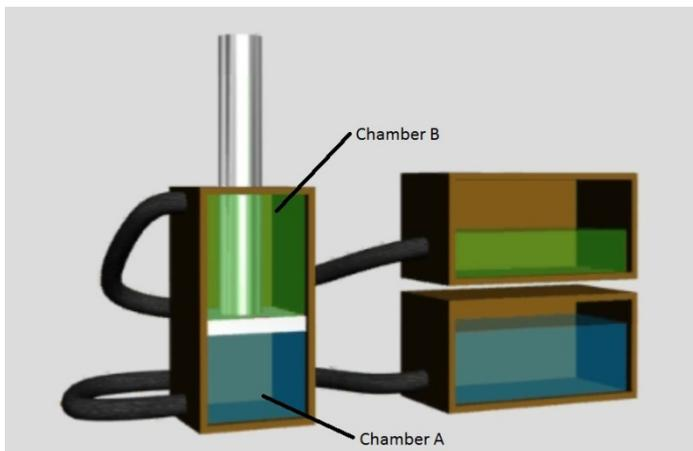
When chamber A (the primary cylinder) is pressurized and chamber B (the secondary cylinder) is open, or vented, the plunger extends and exerts a force that is directed outwardly or in the up direction as shown in the schematic. Conversely, when chamber B is pressurized and chamber A is vented, the plunger retracts and moves inward or down.
