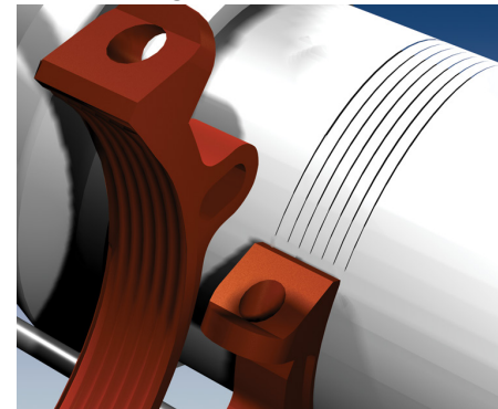
Restraint Ring Tooth Impressions on PVC Pipe.
